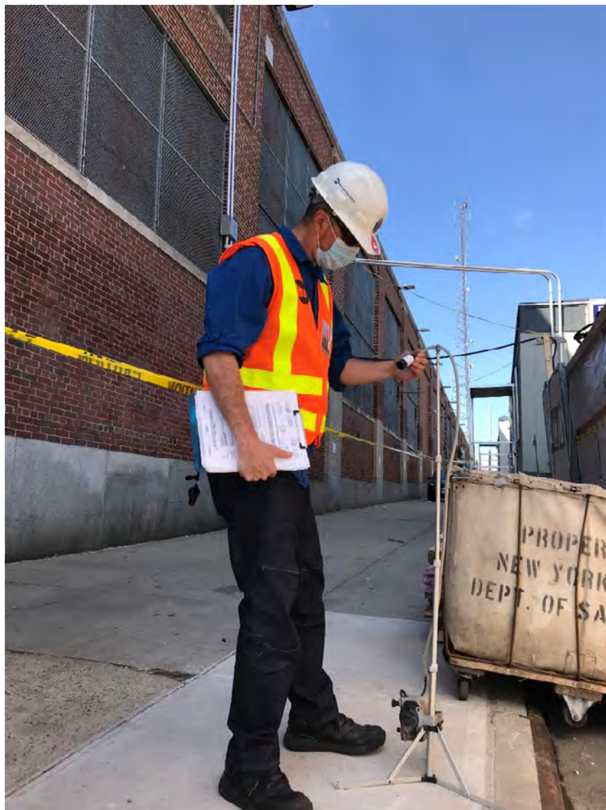
Office of System Safety, Safety Specialist Oscar Suarez, from the Hazard Abatement team, inspects area air sampling equipment at East New York Bus Depot during a window replacement project which also includes asbestos abatement.
